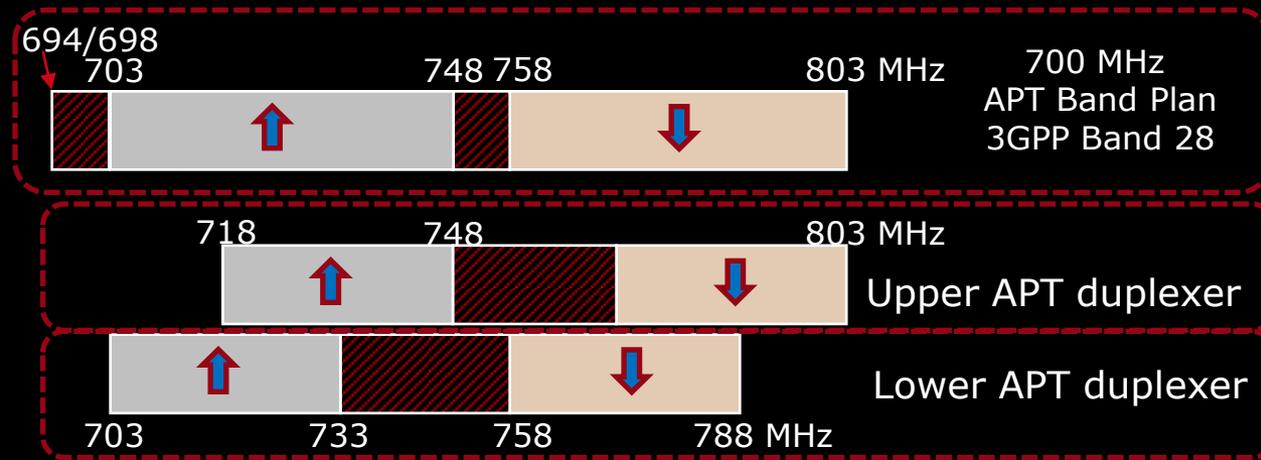
Allow nations to opt for the full bandwidth or restrict to the upper 2x30 MHz or the lower 2x30 MHz to allow for related services in the band and provide overall band plan efficiency
